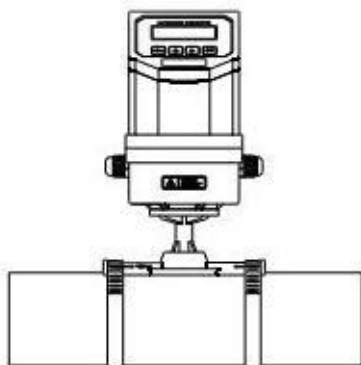
Install on the pipeline
