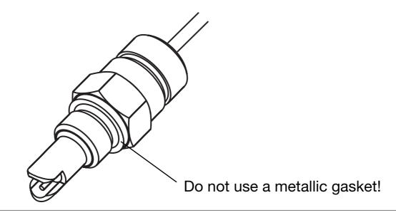
The operating position is generally unrestricted. It must, however, be ensured that the liquid can flow adequately through or arround the sensor (i.e. the conductive electrodes of the sensor must always be completely enveloped by the liquid), and constructional measures must be taken to eliminate interruptions in the flow or gas bubbles.
