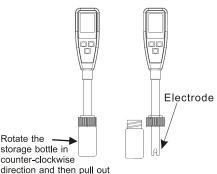
2. Dip the electrode into the test solution. Press " Φ " to power on the meter and tir it to get a stable reading.
