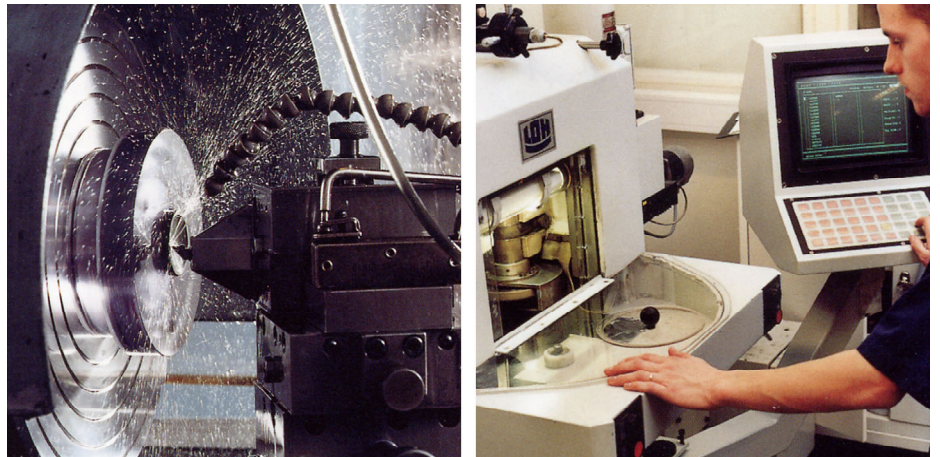
Figure 12.4 LEFT: Diamond turning machine; RIGHT: Lens polishing
