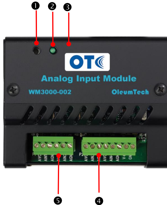
Figure 2-1. Front Components on the Analog Input Module
