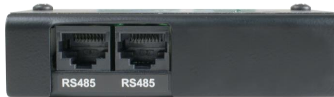
Figure 2-2. RJ-45 Ports on the Top of the Analog Input Module
