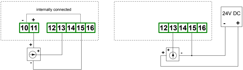
Figure 4.8. Connection of voltage converters
