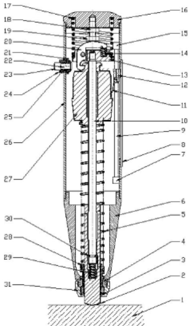
Figure 1 Structure of Test Hammer HT225
