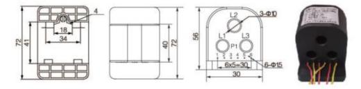
Note:There are six  $\Phi$ 1.5mm RV soft wires lead from the transformer(marked 1,2,3,4,5,6) . S1 is red and S2 is yellow. The outlet must be fixed on P1, and the length of S1,S2 is 3m + 10cm. Primary current flow from P1 to P2.
