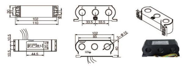
Note: Primary current flow from P1 to P2. The yellow second wiring is A-phase S1, the green is B-phase S1, the red is C-phase S1, and the black is common ground. The outlet length is 2m + 10cm.
