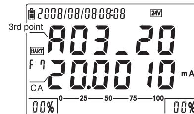
Picture 4–5–7–2: Fixed loop current output
