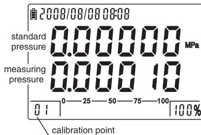
Figure 5–3–2: 1<sup>st</sup> point calibration
