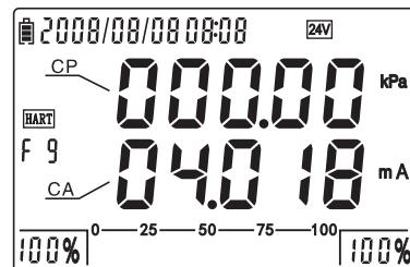
Figure 4-5-9-2: Special calibration interface
