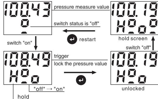
Figure 2-2-5-2 "off" → "on" → "off" dual triggering
