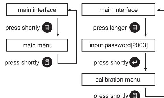
Figure 1–6–1: How to enter into the menu
