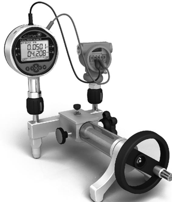
*Remark: If user wants to calibrate the HART type pressure transmitter, please enter into the HART status by pressing
